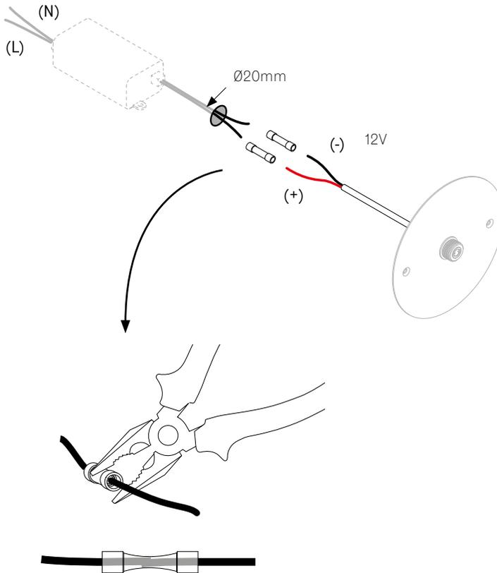
**EN** Connect positive wires to positive 12V and negative wires to negative 12V.
