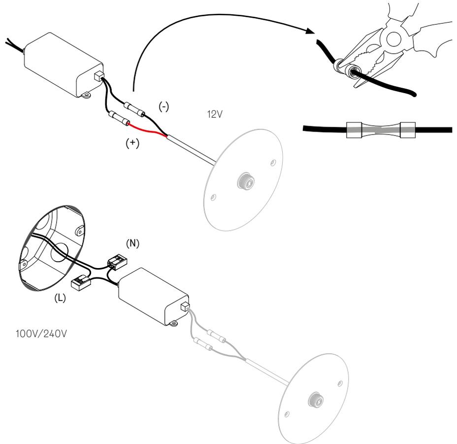
**EN** Connect positive wires to positive 12V and negative wires to negative 12V. Connect live to live (L), neutral to neutral (N).
