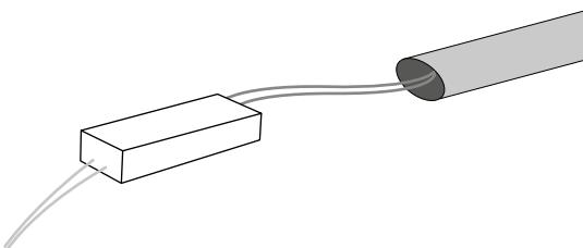
**EN** Connect burial cables to power supplies, ensuring to leave 100-155mm of loose excess burial cable.
