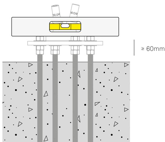
**EN** Do not in-fill this area under the base. Wires must be kept free even after final install.
