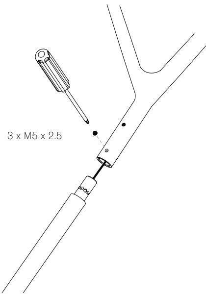
**EN** Refer to specification for branch location. Orient branches as desired, ensuring there is no interference with adjacent branches, pendants or trees.
