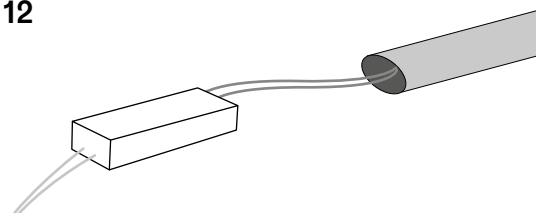
**EN** Connect burial cables to power supplies, ensuring to leave 100-155mm of loose excess burial cable.
