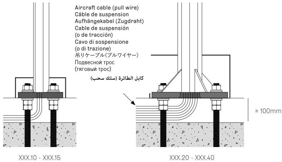
**EN** Do not in-fill this area under the base. Wires must be kept free even after final install.
