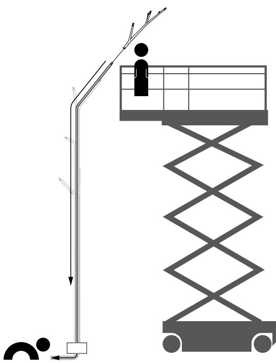
**EN** One person on the scissor lift pushes the wire while the person on the ground pulls the wire.
