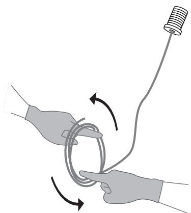
**EN** To avoid kinks, uncoil the coaxial cable in a spool-like manner. Allow the cable to uncoil completely before installing.
