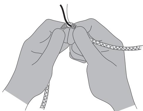
**EN** Using a tool or your hands, pry a small hole in the braided cable to expose the two cables inside. Pull out the insulated cable and the aircraft cable.
