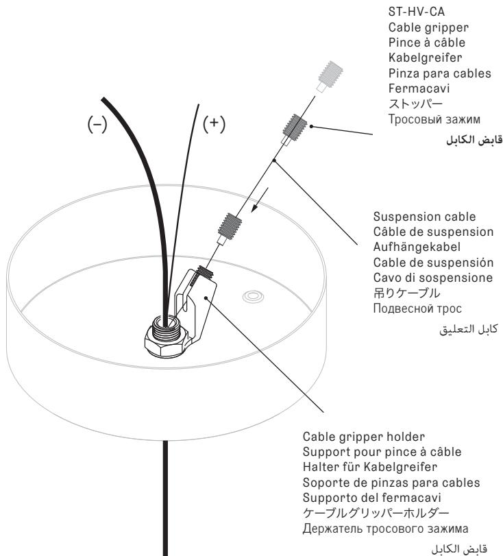
**EN** Thread the cable gripper through the suspension cable and slide the suspension cable into the cable gripper holder located inside the canopy. Push (tighten) the cable gripper against the holder so the cable gripper partially rests in the holder. This suspension cable provides primary support for the fixture.
