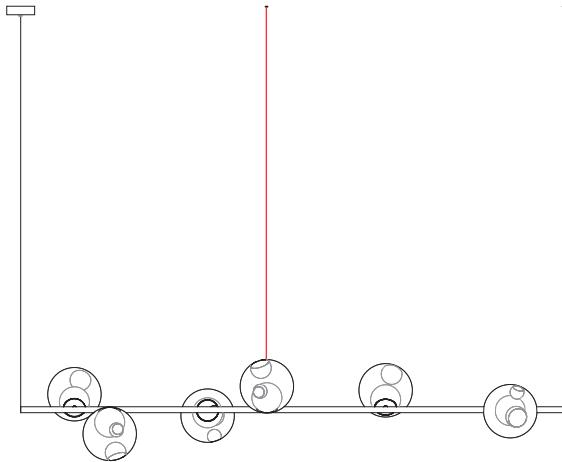
**EN** Required for 1800mm horizontal suspended. The leveling kit should only be attached once the system is installed to the desired height.
