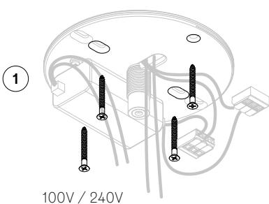
**EN** The client is responsible to ensure fasteners are attached to a robust structural substrate. Max weight 35kg. Connect live to a live (L) and neutral to neutral (N).
