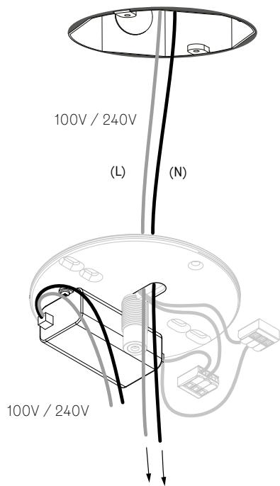
**EN** Feed the live and neutral wires through the slots on the mounting plate.
