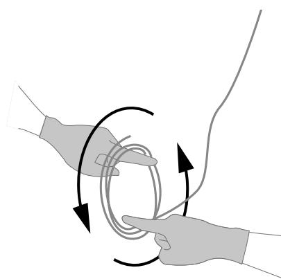
**EN** To avoid kinks, uncoil the sculptural cable in a spool-like manner. Allow the cable to uncoil completely before installing.
