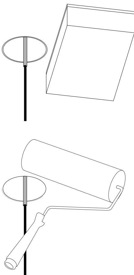
**EN** Using a foam sanding block, sand entire area until the rim and the edge of the operative component are exposed. For long term performance, it is essential that mud is sanded right down to the plastic rim.
