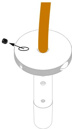
**EN** Loosen the set screw on the copper cap to rotate the cap. There is a channel on the cap for the cable gripper to slide in. Ensure to orient the copper cap with the large opening pointing downward.
