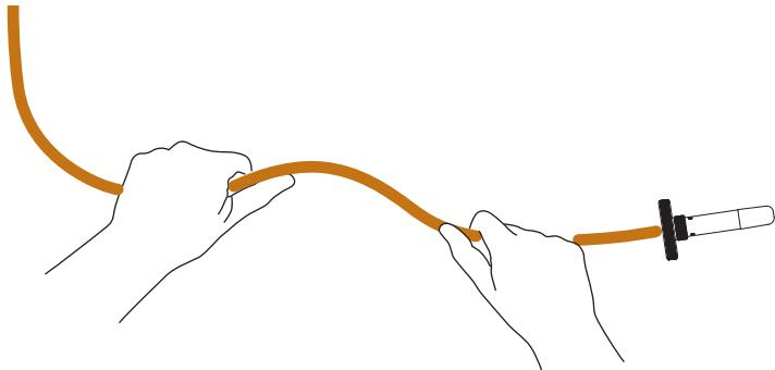
**EN** Compose the copper tubing according to the intended design aesthetic. Note: Once the pendant is added, it will pull the copper downwards. The pendant will try to hang directly below the canopy as the copper is not rigid enough for long horizontal compositions without the addition of pendant anchor kits.
