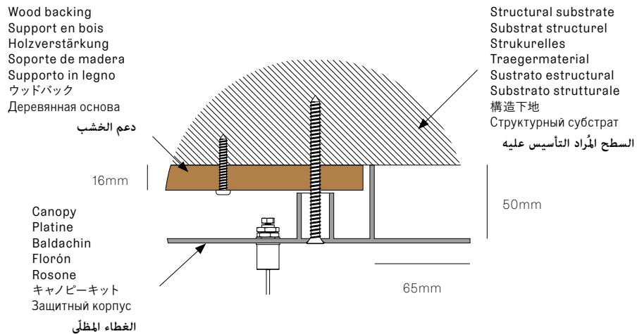
**EN** The client is responsible for providing a robust 16mm marine grade plywood backing to anchor the canopy to the structural substrate. Measure the plywood so that it fits within the internal canopy sidewalls. Refer to canopy spec sheet for canopy dimensions.
