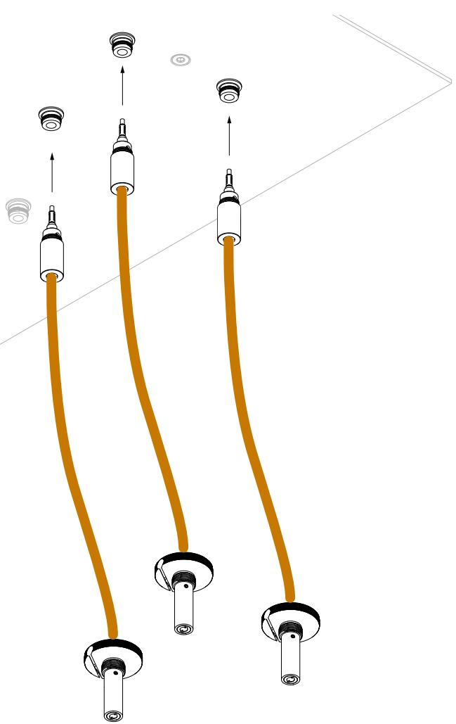
**EN** Locate and install the shortest copper tube for each pendant. These pieces will be the load-bearing length for the pendants.
