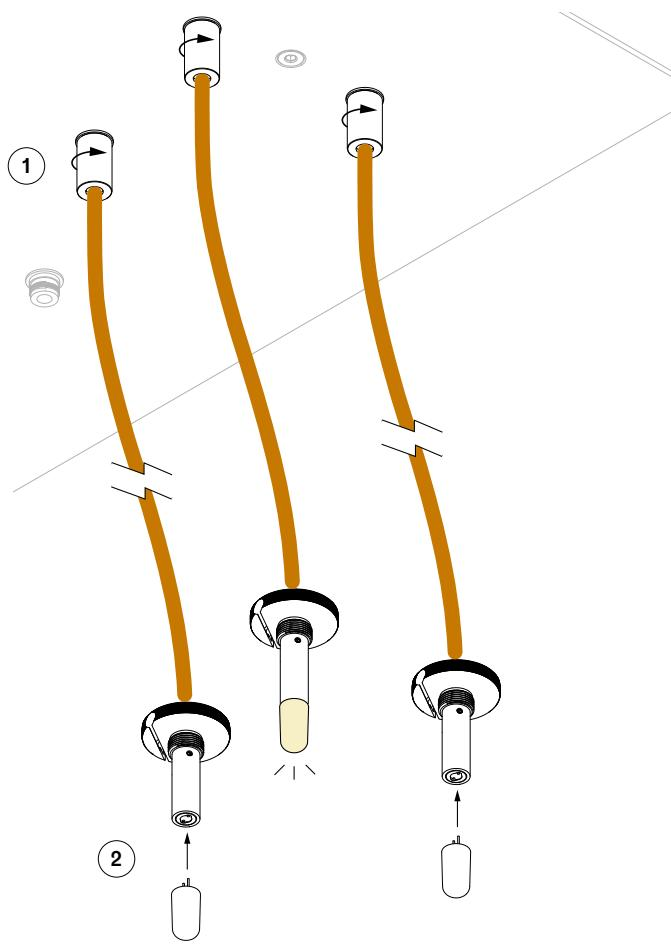
**EN** Check that each lamp is working properly as you go along by turning the power on for every three pendants installed.
