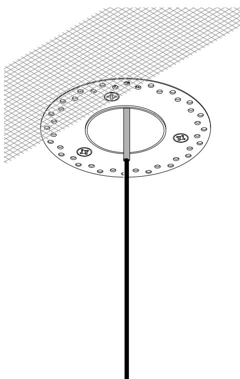
**EN** Mask the coaxial cable off with painters tape to help with cleanup. Tape the mounting plate edges with fiber mesh drywall tape.
