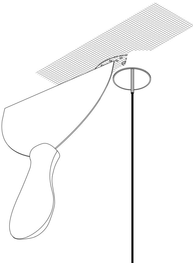
**EN** Use a drywall filler compound to "mud over" the assembly. Use the raised edge to mud up to establish a sharp edge and to avoid getting mud in the indentation. Feather from the center of the mounting plate outwards using a large drywall trowel.
