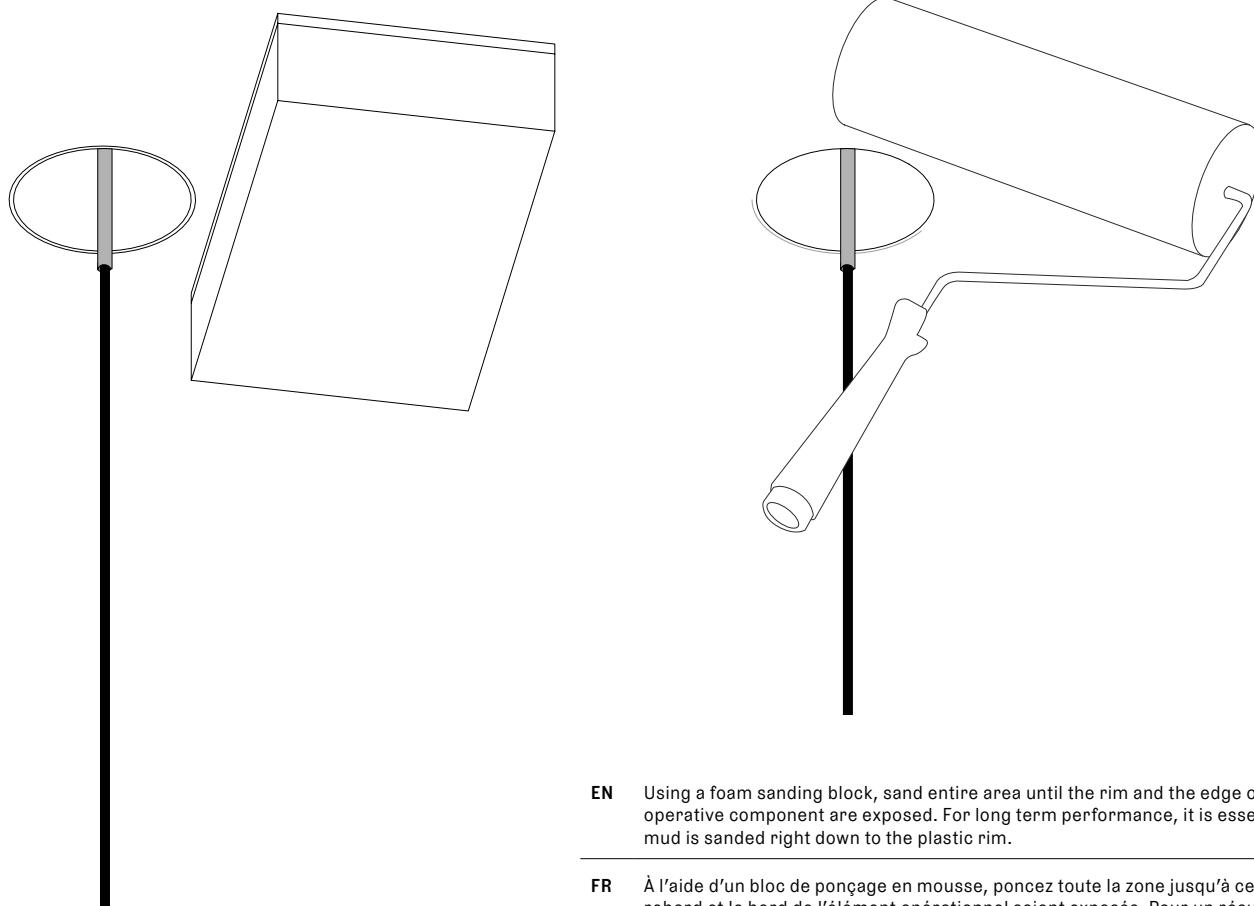
**EN** Using a foam sanding block, sand entire area until the rim and the edge of the operative component are exposed. For long term performance, it is essential that mud is sanded right down to the plastic rim.
