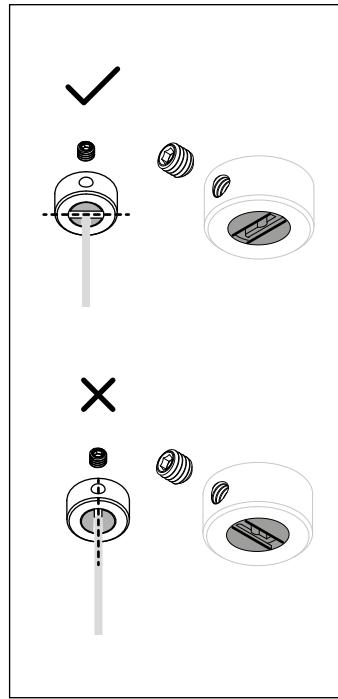
**EN** Do not overtighten! Perform a gentle tug test to ensure the coaxial cable is secure.
