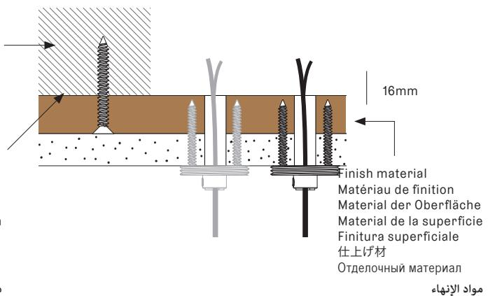
**EN** The client is responsible for providing a robust 16mm marine grade plywood backing to anchor the canopy to the structural substrate.
