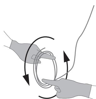
**EN** To avoid kinks, uncoil the coaxial cable in a spool-like manner. Allow the cable to uncoil completely before installing.
