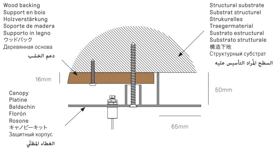
**EN** The client is responsible for providing a robust 16mm marine grade plywood backing to anchor the canopy to the structural substrate. Measure the plywood so that it fits within the internal canopy sidewalls. Refer to canopy spec sheet for canopy dimensions.
