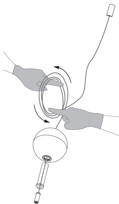
**EN** To avoid kinks, uncoil the coaxial cable in a spool-like manner. Allow the cable to uncoil completely before installing.
