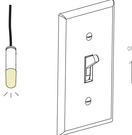
**EN** Check that each lamp is working properly as you go along by turning the power on for every three pendants installed.
