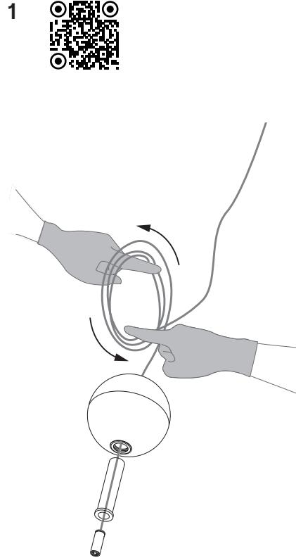
**EN** To avoid kinks, uncoil the coaxial cable in a spool-like manner. Allow the cable to uncoil completely before installing.
