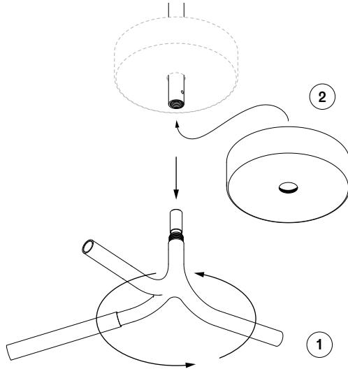
EN Remove AR-C-H to add canopy cover, be careful not to scratch the fixture.
