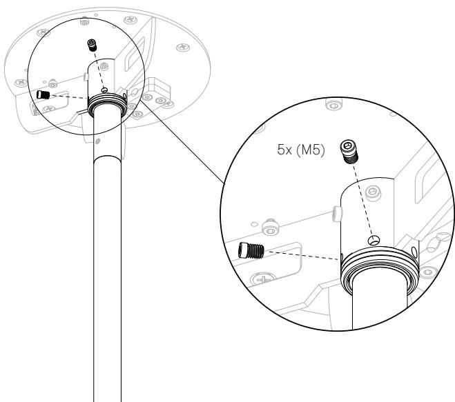
**EN** Tighten screws (x5) on the second row evenly so that all set screws are equally engaged.
