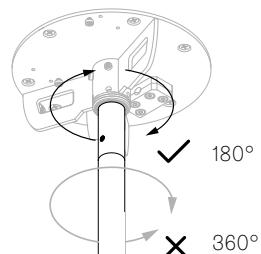
**EN** Check the orientation of the fixture, adjust if needed. Please reference the drawing on the Pendant Specification Sheet for a visual guide.
