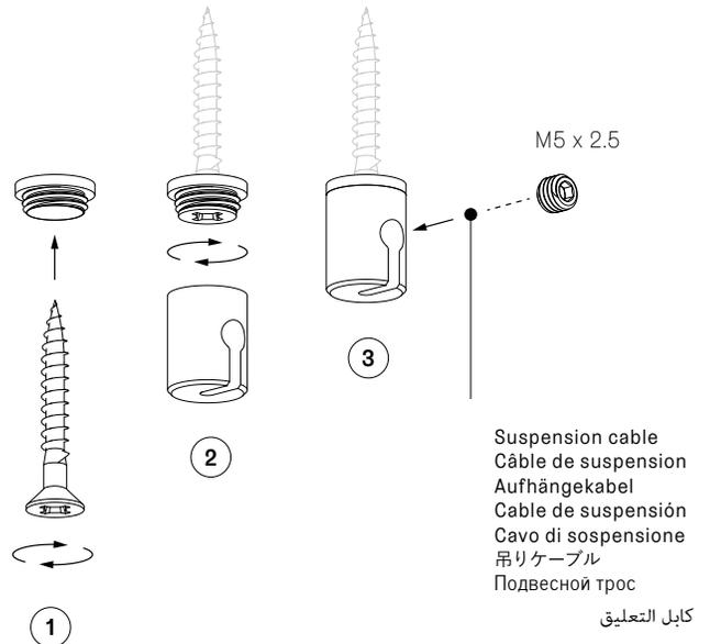
**EN** Once all three pendants are suspended and secured, you have the option to add horizontal dimension by using a jacketed suspension cable and pendant anchor kit (included). Ensure adequate structural support for the weight of the pendant, backing may be required.
