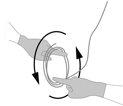
**EN** To avoid kinks, uncoil the coaxial cable in a spool-like manner. Allow the cable to uncoil completely before installing.
