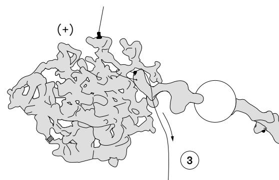
**EN** Find a closed loop on the positive pendant, loosen the griplock cap on the lamp assembly and thread the lamp assembly cable through the pendant.
