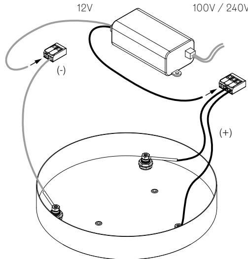
**EN** Connect both positive wires to positive 12V and single negative wire to negative 12V.
