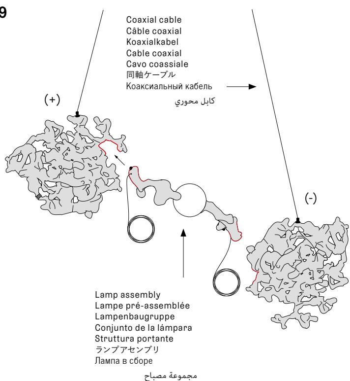
**EN** The lamp assembly must be in contact with the pendants to complete the electrical current that powers the LED.
