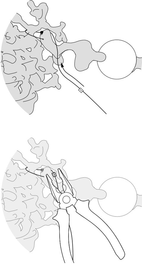
**EN** Slide crimp (included) through the lamp assembly cable and crimp it to the back side of the griplock. This locks the pendant and the lamp assembly in position.
