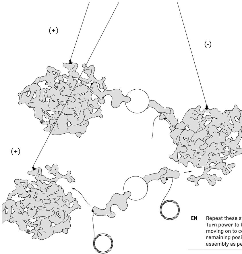
**EN** Repeat these steps to connect the negative pendant. Turn power to fixture on to test the pendant assembly at this stage before moving on to complete the installation. Attach the final pendant to the remaining positive cable and set height and connect the second lamp assembly as per previous steps.
