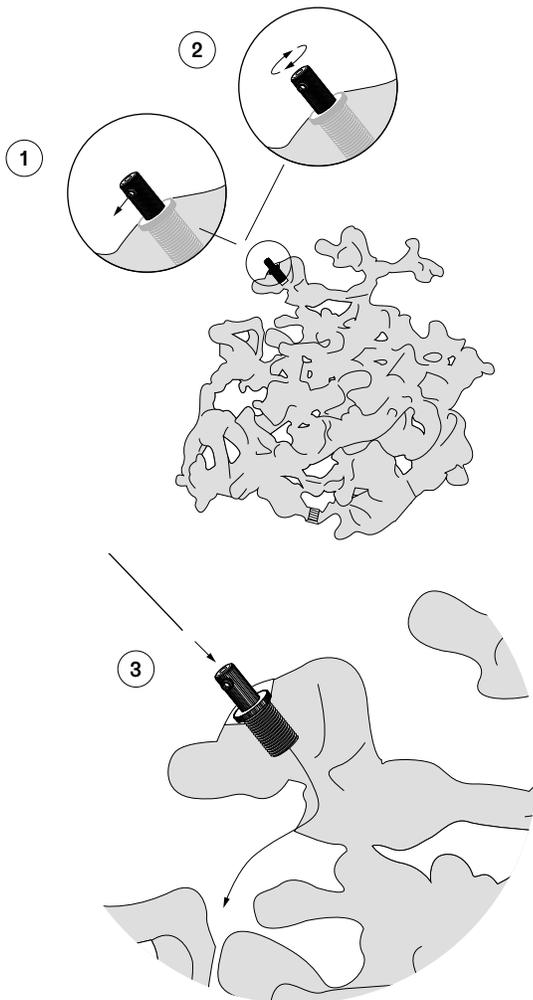
**EN** Bocci recommends wearing gloves during the installation. The aluminum pendant may be sharp to handle. Loosen the set screw and griplock cap located on the pendant that will be connected to a positive cable. Slide the cable through the griplock to set the height.
