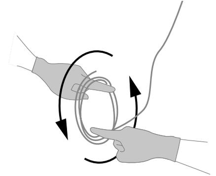
**EN** To avoid kinks, uncoil the coaxial cable in a spool-like manner. Allow the cable to uncoil completely before installing.
