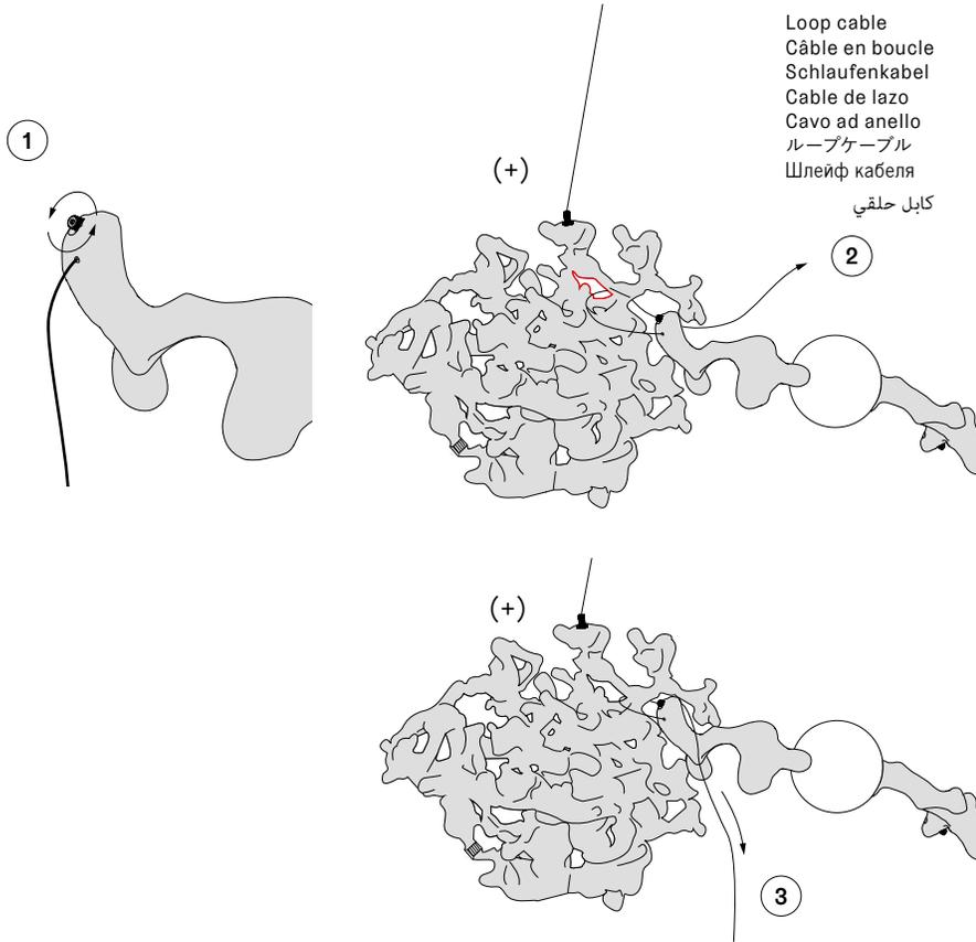
**EN** Find a closed loop on the positive pendant, loosen the griplock cap on the lamp assembly and thread the lamp assembly cable through the pendant.
