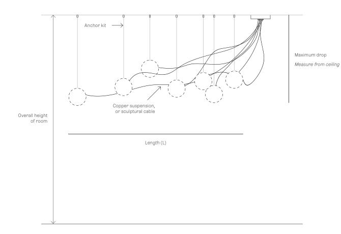
Sculptural cable or a copper suspension system in a cluster configuration with pendant anchor kit.
